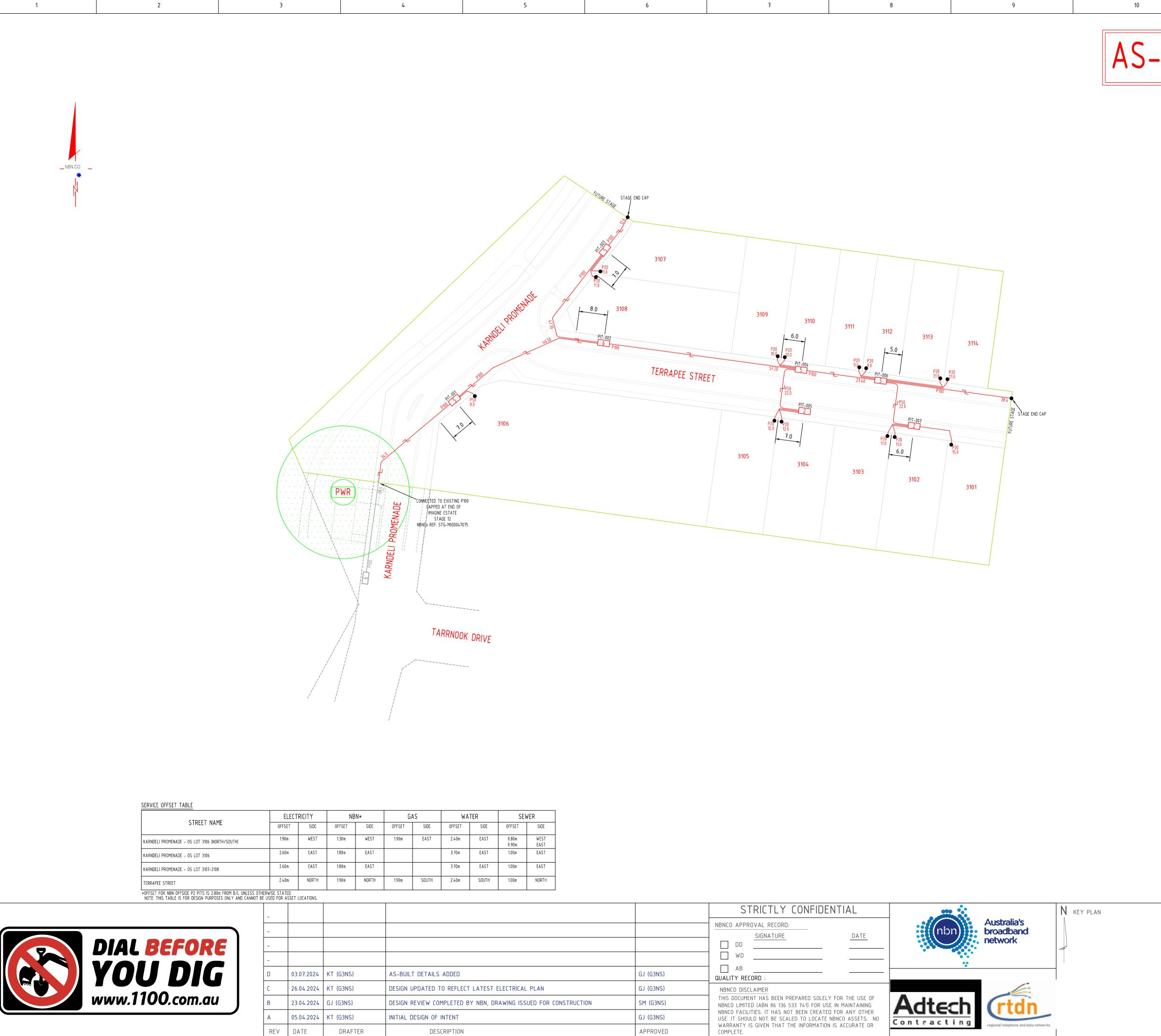
PIT LEGEND Shared Trench Symbol PIT-ID Service Drop Access Pit 650mm(L) x 280mm(W) x 565mm(D) PIT-ID Network Boundary/Local Network Pit  $700 \text{mm}(L) \times 450 \text{mm}(W) \times 650 \text{mm}(D)$ PIT-ID Distribution/Local Network Connection Pit 1360mm(L) x 555mm(W) x 650mm(D) PIT-ID Distribution/Local Network Connection Pit 1360mm(L) x 555mm(W) x 860mm(D) PIT-ID Fibre Distribution Hub Pit 2000mm(L)  $\times$  555mm(W)  $\times$  900mm(D)
