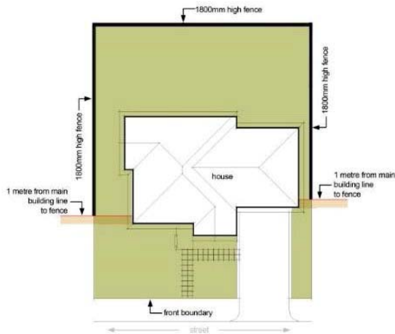
Depiction of typical boundary fencing location
