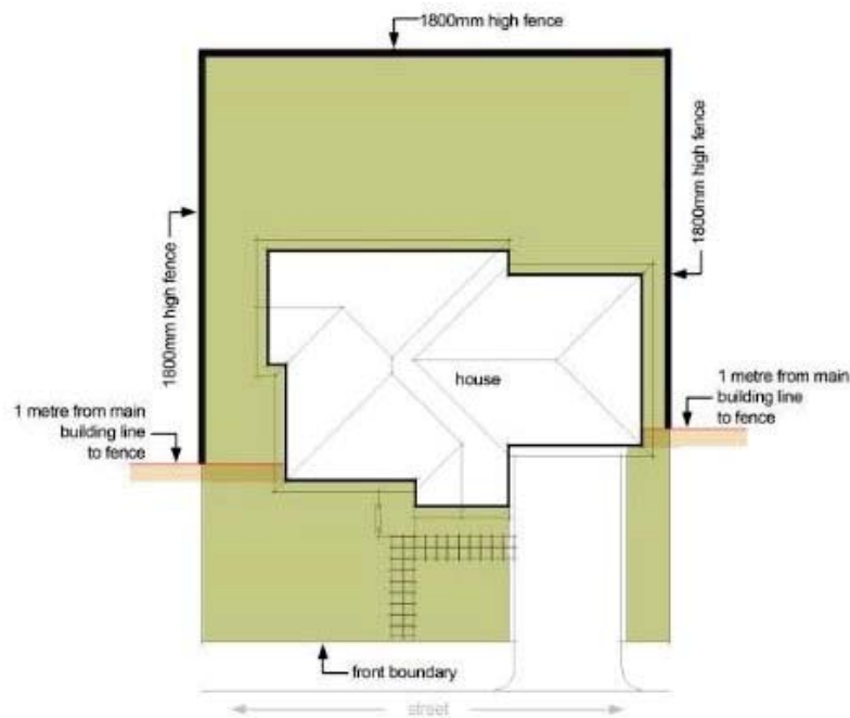
Depiction of typical boundary fencing location
