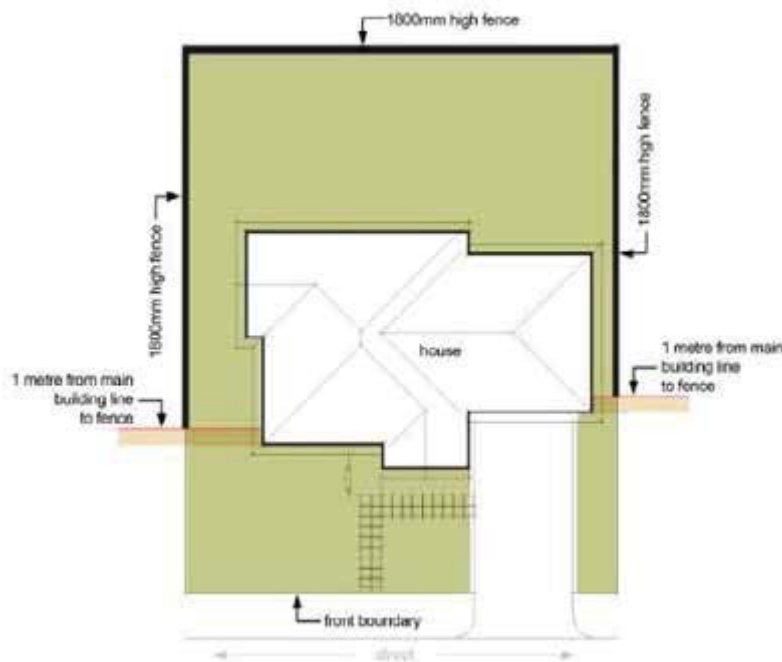
Depiction of typical boundary fencing location
