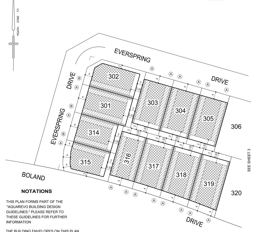
THE BUILDING ENVELOPES ON THIS PLAN ARE SHOWN ENCLOSED BY CONTINUOUS THICK LINES
