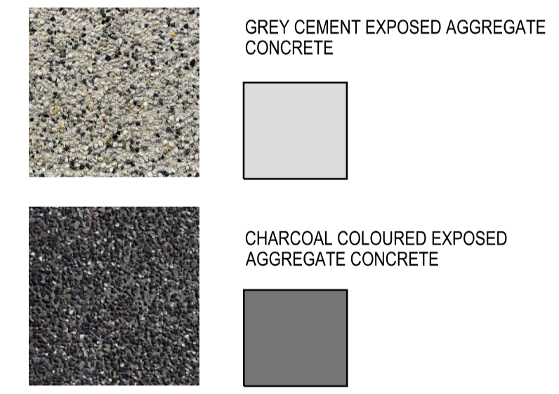
FEATURE EXPOSED AGGREGATE PAVING ALL WORKS GENERALLY IN ACCORDANCE WITH HUME SD307
