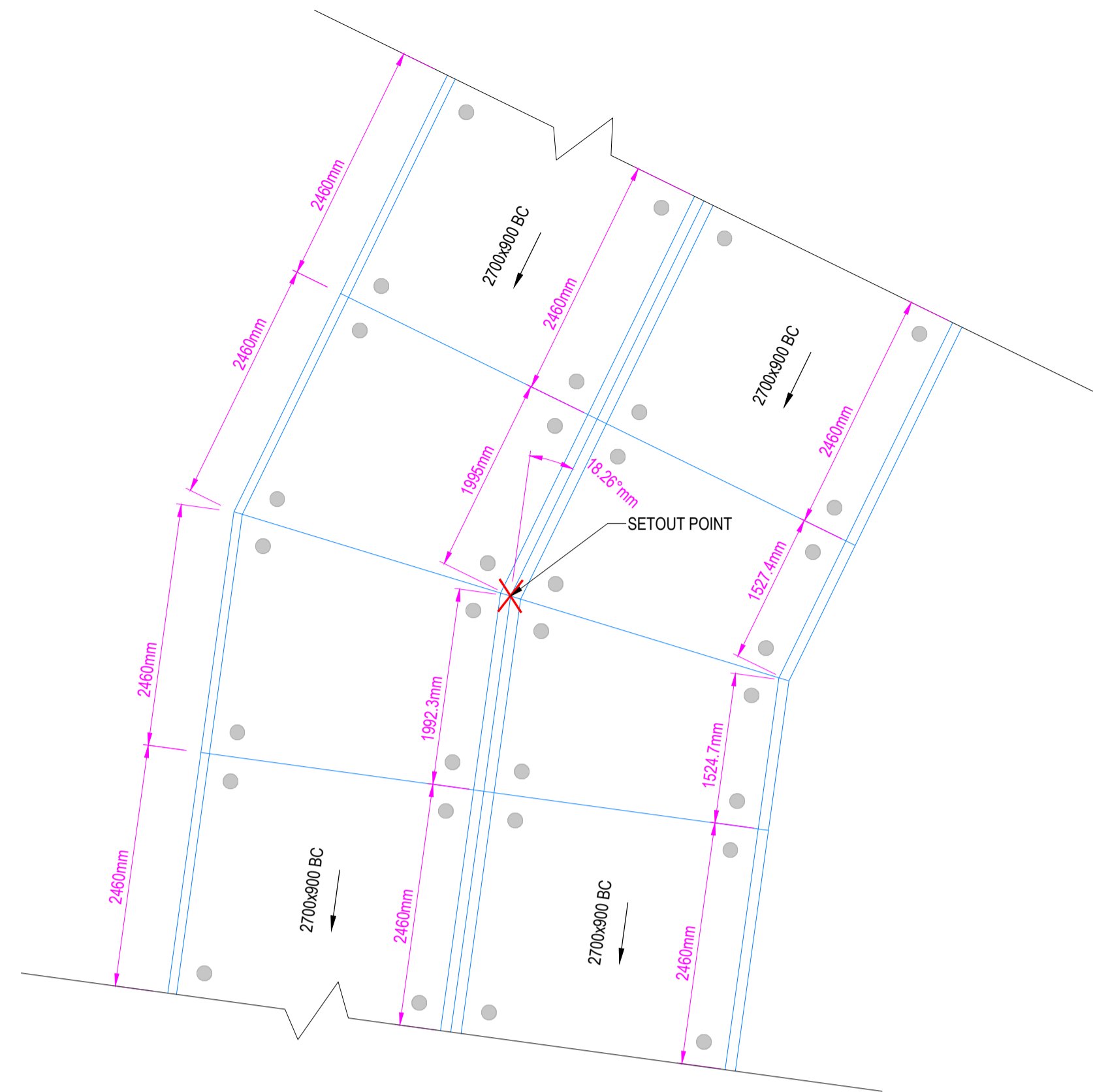
'SKEWED' BOX CULVERT DETAIL (TP5) PLAN VIEW 1:50
