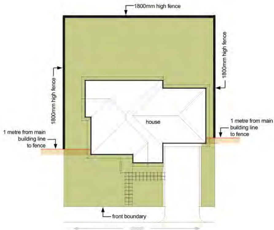
Depiction of typical boundary fencing location
